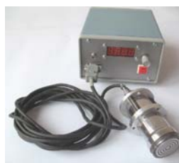
Fig. 1 General view of the electromagnetic non-destructive measuring unit and remote measuring transducer for determining level of CFx fluorination
